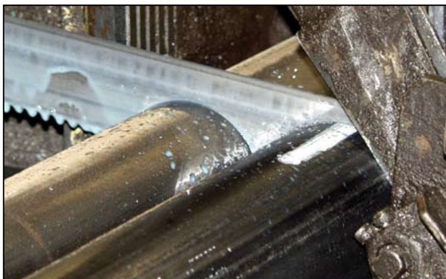
Saw Blade Going Through A Round Bar
